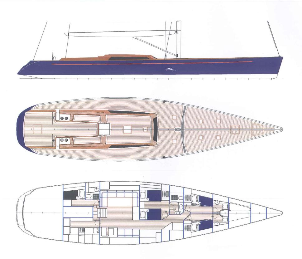
PRELIMINARY OUTBOARD PROFILE **DECK PLAN & INTERIOR LAYOUT**
