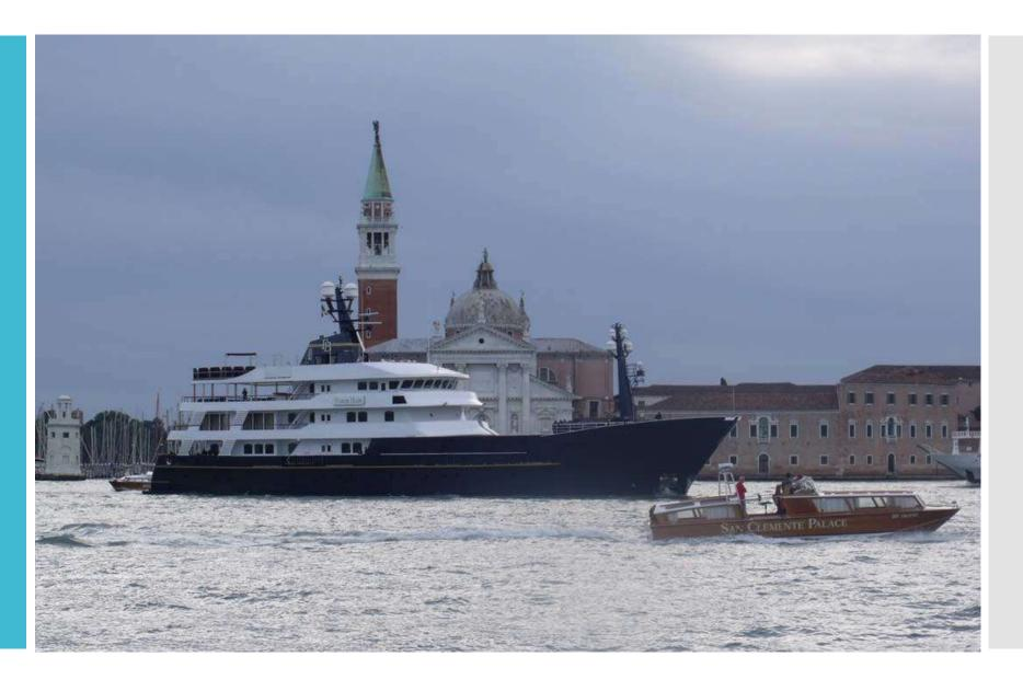
Built by Danish shipyard Royal Denship in 2002, FORCE BLUE was fully redesigned in 2006 with a stunning new interior decor from Celeste Dell'Anna. Built in aluminium with a steel hull, FORCE BLUE cruises comfortably at 14 knots in all conditions. Designed to offer the ultimate charter experience, FORCE BLUE's award-winning crew and captain are renowned for their professionalism..
